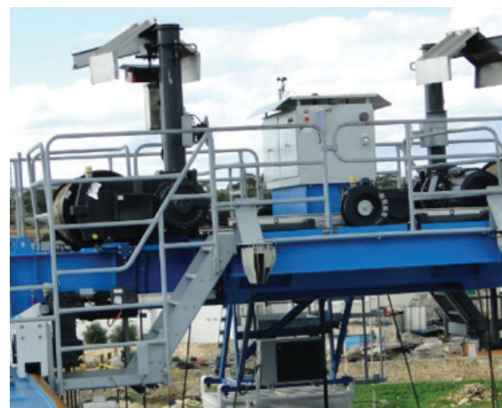
Service hoist for typical 8W RTG trolley (two jibs)
