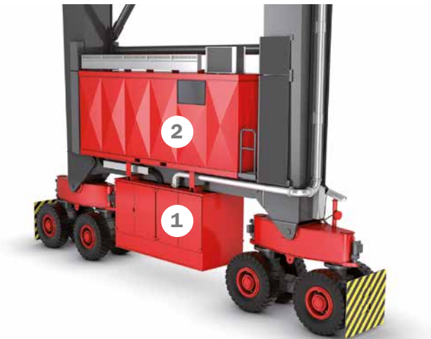
Figure 2. The diesel fuel saver is retrofitted in the genset enclosure (1) while the necessary modifications to the electrical systems are made in the e-house (2) above it. Some software modifications are also done at the same time.
