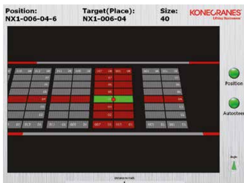
Figure 15. Yardscreen uses a graphical interface to show current crane position and locate container slots.
